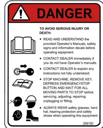
Wear Personal Protective Equipment (PPE) – know how to use the protective equipment when operating the machine. Hard hats, protective glasses and face shields, protective shoes, gloves, reflector type vests, and ear protection are types of equipment that may be required.
