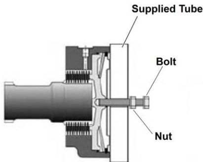
Position the supplied tube with the hole centered over the brake access hole. Insert the supplied bolt / nut through the hole in the tube into the brake housing.
