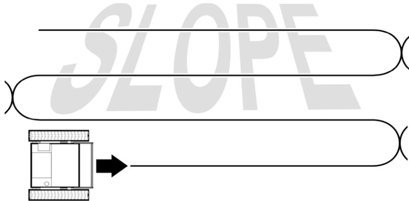
The preferred cutting direction on slopes is to cut along the slope and not up and down. Mowing in this manner could also help reduce erosion. Always use three point turns at the end of each pass. Remember to vary mowing pattern over time to avoid the creation of ruts in the terrain from.
