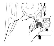
Once the engine is running, verify the Check Engine and Low Engine Oil Pressure warning lamps on the console are OFF. If they are NOT off, stop the engine immediately and have a qualified technician rectify the problem.
