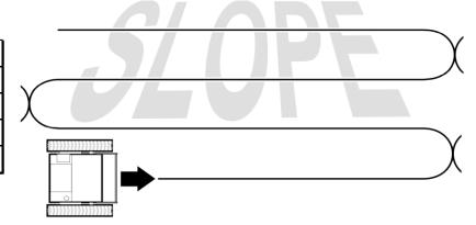
The preferred cutting direction on slopes is to cut along the slope and not up and down. Mowing in this manner could also help reduce erosion. Always use three point turns at the end of each pass. Remember to vary mowing pattern over time to avoid the creation of ruts in the terrain from.
