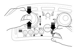
Push the Engine Start toggle switch forward to engage the starter. Release when the engine starts.
