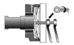
Tighten the nut while holding the bolt preventing it from turning. As the nut is tightened\* the brake is released, continue tightening the nut until the motor turns freely. The brake on that side of the machine is released. Repeat on the other side of the machine.
