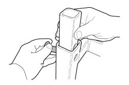
Insert the pins through the machine frame and jack tube; secure the pins in the tube with the clip.
