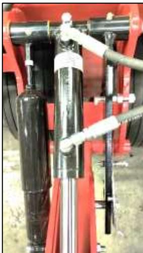
As required, change the position of the shock absorber and the deck lock so that the hoses are routed over the deck lock and not the shock absorber as shown. See the installation instructions within kit 670038 for more information.
