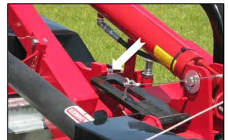
A deck latch plate correctly positioned during Pro Lift-N-Turn operation.
