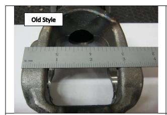
Progressive Turf Equipment Part #210231 Used on input PTO shaft Part #210230 Outside measurement at cross: Approximately 3½"
