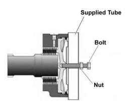
Tighten the nut while holding the bolt preventing it from turning. As the nut is tightened\* the brake is released, continue tightening the nut until the motor turns freely. The brake on that side of the machine is released. Repeat on the other side of the machine.
