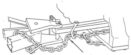
• Install a safety chain as shown. After attaching the safety chain, make a test run to the left and right for a short distance to check for proper adjustment. Readjust to eliminate a loose or tight chain.
