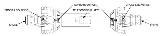
\* Inner & outer guards must be rotated to align holes for accessing telescoping shaft grease fitting.
