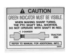
DISENGAGE PTO SHAFT
