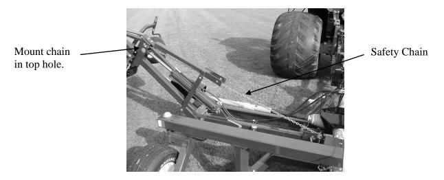
Two holes on frame to anchor the safety chain.
