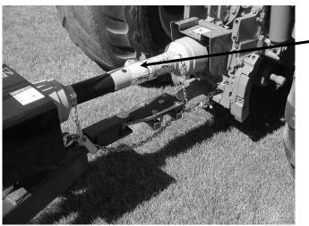
Proper setup will allow you to see the grease zerk on PTO shaft.
