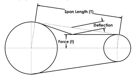
The recommended force to deflect the belt is a minimum of 4.9 lbs. to a maximum of 7.3 lbs.
