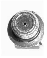
When reconnecting the quick disconnects to the tractor, be sure that both ends are clean. Dirt in the hydraulic system can block the orifice in the line throttle valve or even score the cylinder tubes.
