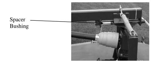
This spacer bushing can be mounted on either side of the wing deck swivel.
