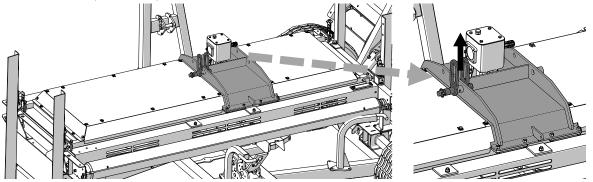
If overhead lifting facilities are not available, a fork-lift can be used to remove the decks from shipping brackets. This may require removal of the wing frame to properly access the deck (Domestic truck shipping only).
