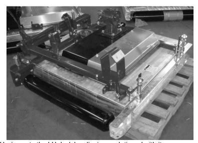
8) Place the LH wing onto the LH deck by aligning each tie rod with its corresponding mount point.
