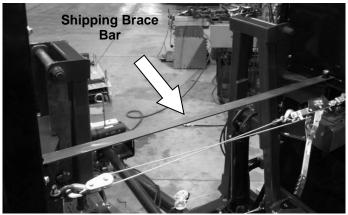
3) Tighten the device until enough tension is relieved from the shipping brace bar. Remove the wire securing the flat bar to the wing, and the flat bar itself.
