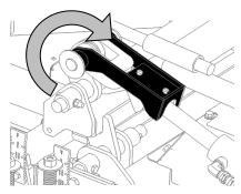
Cylinder Stop Engaged for mowing
