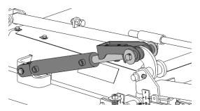
20) Connect the outer wing lift circuit to a hydraulic power source (tractor or power pack) and extend the cylinders until they align with the mounting brackets on the lift pivot bar. Connect cylinder and lift stop to lift pivot bar using pin & hardware on cylinder as shipped.
