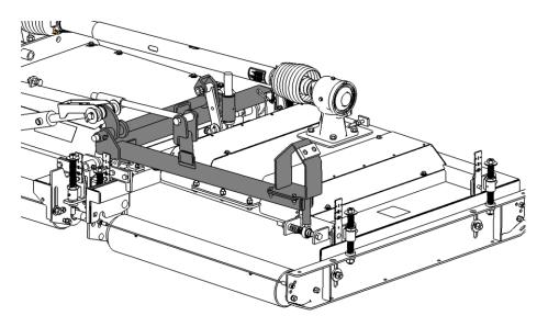
**Outer Wing Deck Installed onto Main Wing Deck**
