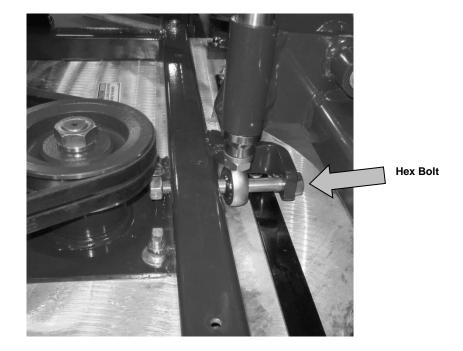
9) Remove the 5/8" x 6 hex bolt from the deck frame and install it through the lift shaft tie rod.
