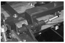
16) Cut all plastic ties securing the wing stop rod. Remove the 5/8" hex bolt and lock nut from the upright brackets on the Outer Wing and fasten the stop rod in place between the mounting brackets.
