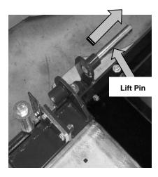
13) Move the Outer Wing Deck towards the main wing deck until they contact the front and rear plastic bumpers on the wing deck. Align the outer wing frame bushings above the main wing frame bushings.
