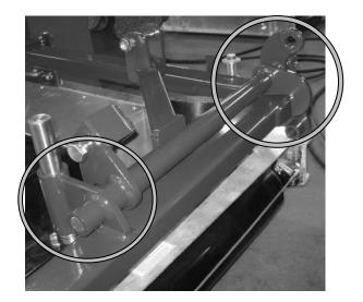
5) Remove the 5/8" x 8.5" bolt, springs, bushing and hardware from the deck frame in order to remove the wing.
