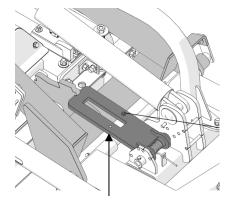
Lock plate engaged during Pro Lift-N-Turn operation.
