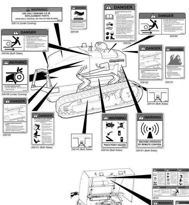
Decal part numbers are shown below the respective illustrations. Always replace damaged or illegible decals. Contact your dealer for a replacement.
