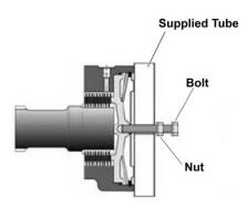
Position the supplied tube with the hole centered over the brake access hole. Insert the supplied bolt / nut through the hole in the tube into the brake housing.
