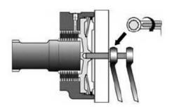
Tighten the nut while holding the bolt preventing it from turning. As the nut is tightened\* the brake is released, continue tightening the nut until the motor turns freely. The brake on that side of the machine is released. Repeat on the other side of the machine.
