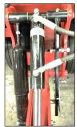
As required, change the position of the shock absorber and the deck lock so that the hoses are routed over the deck lock and not the shock absorber as shown. See the installation instructions within kit 670038 for more information.
