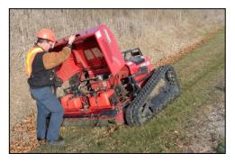
A 747 cc, twin cylinder air cooled Kohler engine – sized for productivity, chosen for fuel economy and reliability, provides power to the mower deck and the variable speed hydrostatic track drives.
