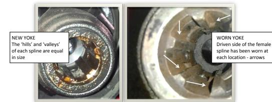
For these same reasons, it is also a good idea to periodically remove, clean and grease all PTO shaft connections to each gear box when performing scheduled service on the PTO shaft.
