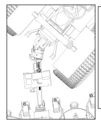
When turning or starting to climb a hill, the input shaft must be able to collapse to accommodate the shorter distance between the tractor and mower.
