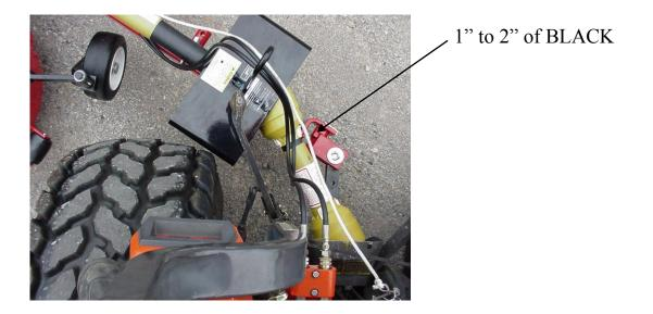
**<u>NOTE</u>**: This is not the worst condition. Making turns while the tractor is angling up a hill will cause the PTO shaft to collapse even more. The operator should avoid making sharp turns on uneven ground.
