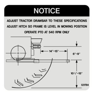
Drawbar should be adjusted so it is 14" to 15" from the centerline of the draw pin hole to end of PTO shaft. This is critical for proper PTO shaft operation.
