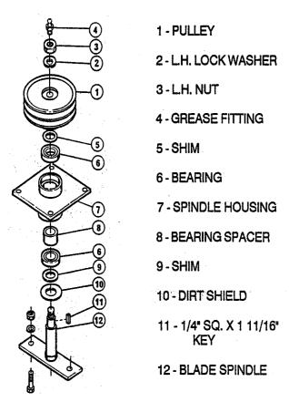
If bearings are being changed, be sure to check bearing spacer for wear. If wear is noticed, insert new spacer. This is critical because if spacer is short by only .010", the top bearing will start to bind and will result in premature failure.
