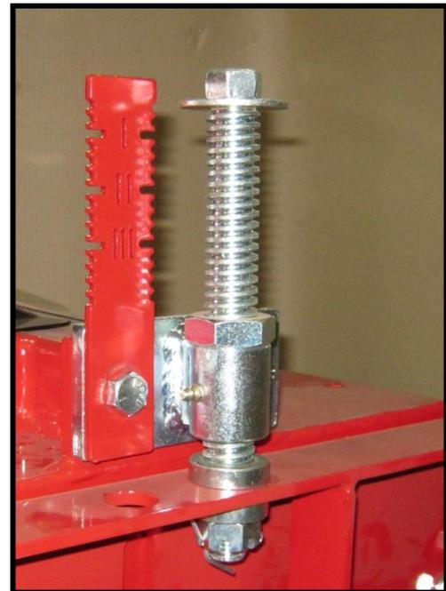
Photo shows the new height adjustment gauge and metal adjustment bushings. The rear plate is shown. The front plate is identified with an **F** cut into the plate.
