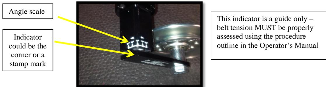
Prior to the expense of replacing a belt, look at the tensioners and locate an angle scale printed on one corner of the housing and a corresponding stamp mark on the arm.
